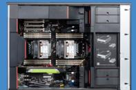
The ThinkStation P900 and P700 Series are built to support dual Intel Xeon scalable processors and up to the new NVIDIA Quadro RTX 8000 graphics inside.
